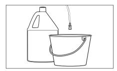
**Step 2** Fill a container with Karcher detergent. Place the filter end of detergent suction tube into the container.
